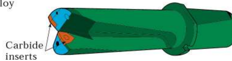
(g) Drill with indexable carbide inserts
