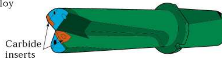
(g) Drill with indexable carbide inserts
